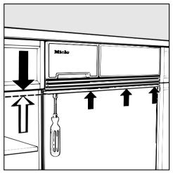
Adjustment range for the adapter strips: max. 10 mm upwards (see arrows in the illustration).
